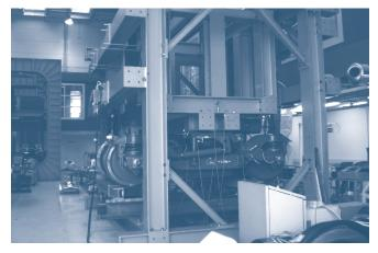
line: calibration of the measurement system (EN50317, RFI/DI/TC.TE/ ST.TE 74D).
